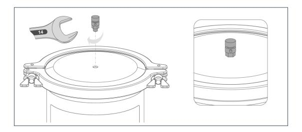
1. Screw the air vent tightly onto the top of the cover.
